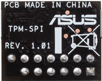
The TPM-SPI card securely store keys, digital certificates, passwords, and data. It helps enhance the network security, protects digital identities, and ensures platform integrity.
